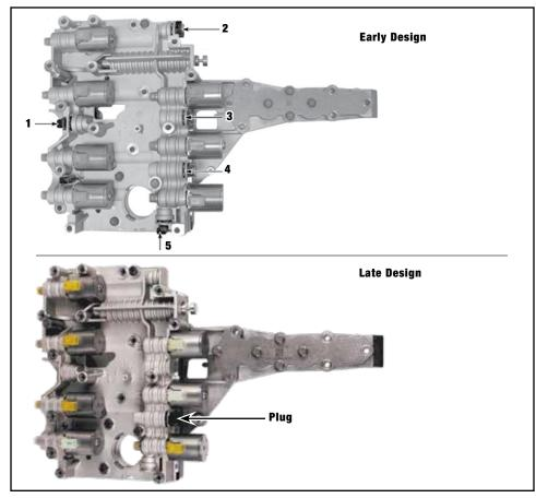
5R110W solenoid body **F05R110** is serviced without any pressure switches. Your original solenoid body may have one or five pressure switches depending on model year. The computer on these vehicles was never programmed to monitor the pressure switches and Ford removed them in late 2004. The later solenoid body may have one pressure switch with no wire going to it. In this application it is only used as a plug with the remaining four holes cast over.
